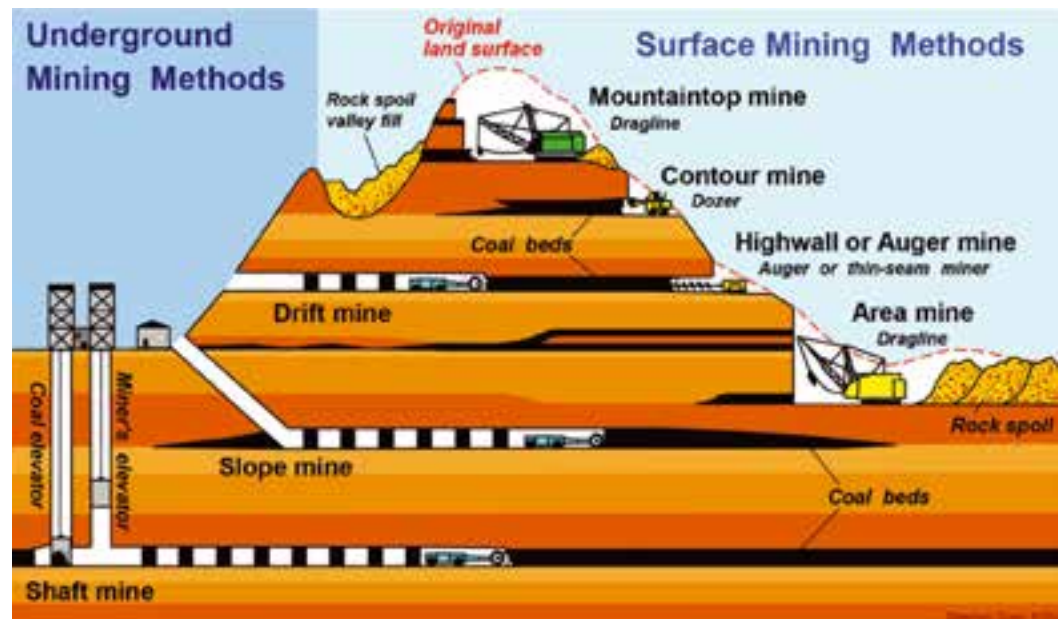
Different Types of Mining. Source: Stephen Greb, Kentucky Geological Survey, University of Kentucky.
