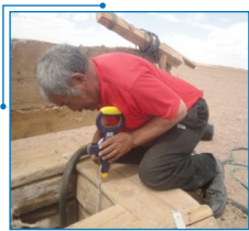
Water level measurement by handmade dipper
