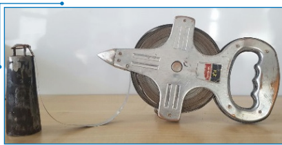
Handmade water level dipper
